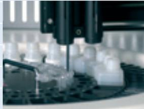
2 heated pipetting needles
