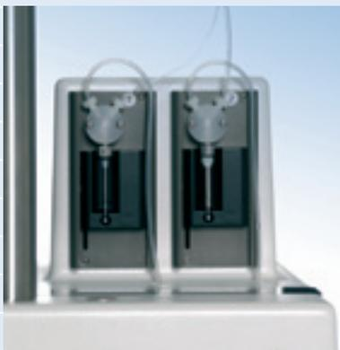
2 independent liquid channels for precise pipetting of reagent and sample
