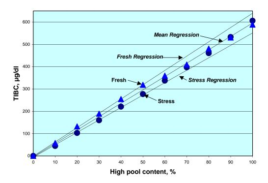
Conclusion: Based on a 10% deviation limit the TIBC method is linear up to at least 500  $\mu$ g/dl. Fresh reagents tend to slightly underestimate high TIBC concentrations, while stressed reagents tend to slight overestimation. A mean regression of fresh and stressed reagents show excellent linearity up to 600  $\mu$ g/dl.
