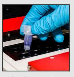
> Incubate the tube in the HumaLoop T heating unit for 5 min at 90°C.
