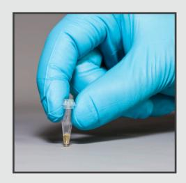
> Tap the reaction tube point down on a hard surface several times until the reaction mixture is collected at the bottom.
