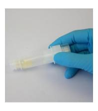
Attach the cap to the nozzle of the Injection Cap. Avoid touching the nozzle!
