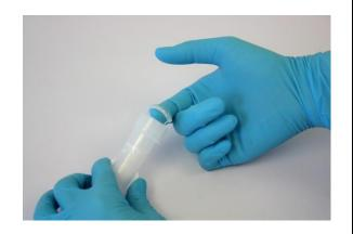
Connect the Heating Tube to the Adsorbent Tube by screwing to release the solution into the Adsorbent Tube.
