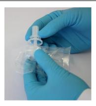
Hold the Adsorbent Tube upside-down and connect the Injection Cap by pushing once and then screwing.
