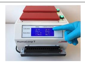
Load the Heating Tubes into the heating block of HumaLoop T and close the lid. Press the Start/Stop button, to start 5 minutes of incubation.
