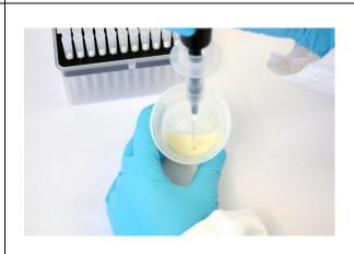
Transfer  $60\mu L$  of sputum into the respective Heating Tube.
