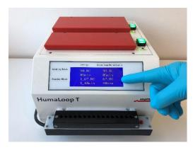
Place the tubes into the reaction block and close the lid. Press the Start/Stop button.
