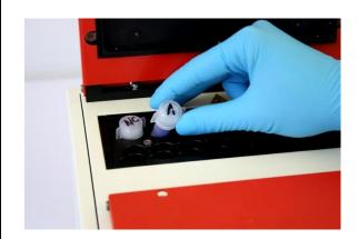
Remove the Heating Tubes immediately after the incubation has finished. This is indicated by an audible signal. Let them cool down for 2 minutes, then mix again 3-5 times.
