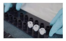
Tap the Adsorbent Tubes to loosen the white powder.
