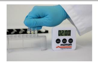
Invert the reaction tubes 5 times to mix the content.
