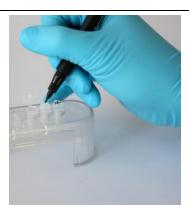
Dispense  $30\mu L$  of PC into a Reaction Tube. Close the cap and mark it respectively.
