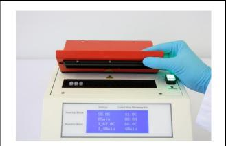
After the audible signal indicates that the amplification is finished, take the Reaction Tubes out of the reaction block and put them into the fluorescence detection unit. Turn on the UV Light by pushing the red button.
