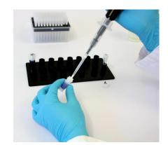
Transfer  $60\mu L$  of NC into the respective Heating Tube.
