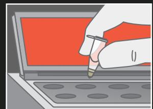
Incubate the reaction tube in the HumaLoop T reaction unit or HumaTurb A for 45 min at 67°C.
