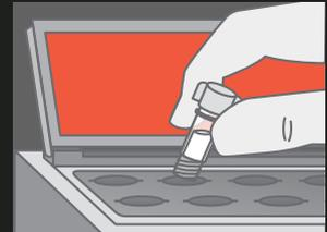
Incubate the tube in the heating unit of HumaLoop T or HumaHeat for 5 min at 90°C.
