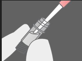
Transfer 60  $\mu$ l sputum with Pipette-60 into the heating tube.
