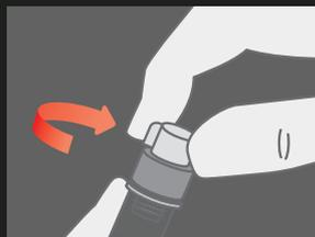
Screw the heating tube onto the adsorbent tube.
